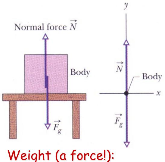
•The internal forces within the table supply a normal force, which is directed normal to the surface of the table, i.e., up.
