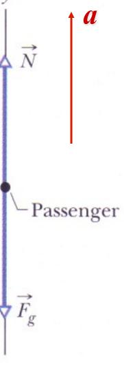
•The scale reading is equal to the normal force on the passenger from the scale.
